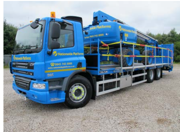
Hi Vis Handrail & Driver Fall Protection
